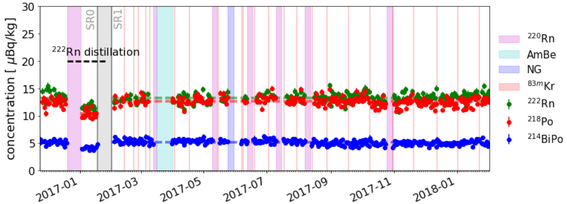
Figure 6.5. Radon monitoring of the rates from ^{222}\text{Rn} (green), ^{218}\text{Po} (red) and ^{214}\text{BiPo} (blue) in order to constraint the rate of ^{214}\text{Pb} , the most dominant background for dark matter search due to its \beta -decay nature. Adapted from [223].
