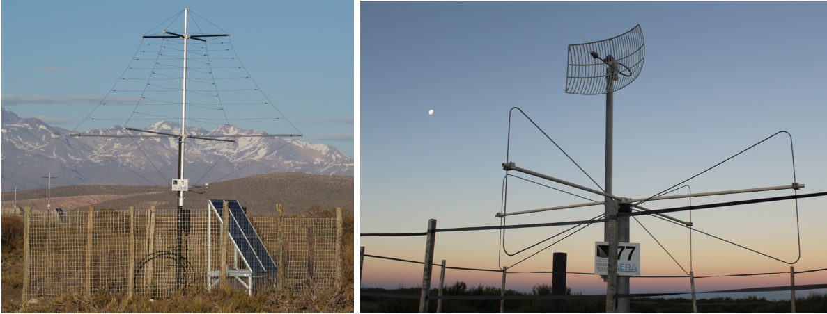
Figure 3.2: Antenna types used for AERA. (Left) A logarithmic periodic dipole antenna used in AERA phase I. Picture from [80]. (Right) A butterfly antenna used in AERA phase II and III.
