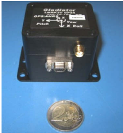
Figure 1-7. Landmark™20 eXT MEMS-based IMU
