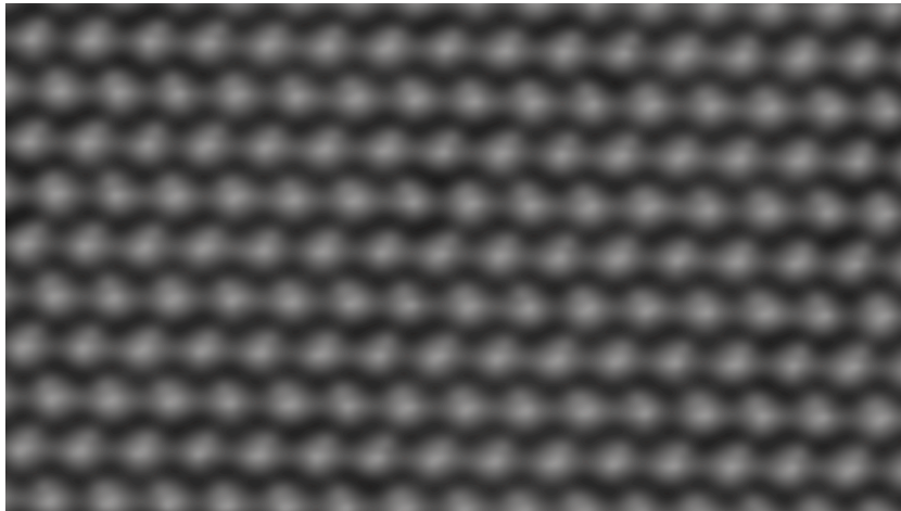
Figure 9.5.: Render of a simulated AFM image of a TPT-SAM. Grayscale encoding from black to gray for the height profile from lowest to highest z-coordinate.
