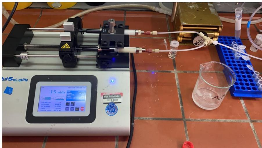
**Figure 75:** Foto of the flow setup showing the syringe pump with the two installed glass syringes, a T-piece and the reactor on the right. The Eppendorf tubes were used to take samples. The bottom Pickering emulsion (PE2) contained the enzyme.
