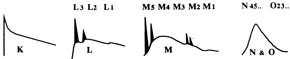
Figure 6 Schematic illustration of K, L, M, N and O edge shapes; the "white lines" sometimes detected on L and M shells are shown as shaded peaks at the edge onsets. In all sketches the background shape has been omitted for clarity.
