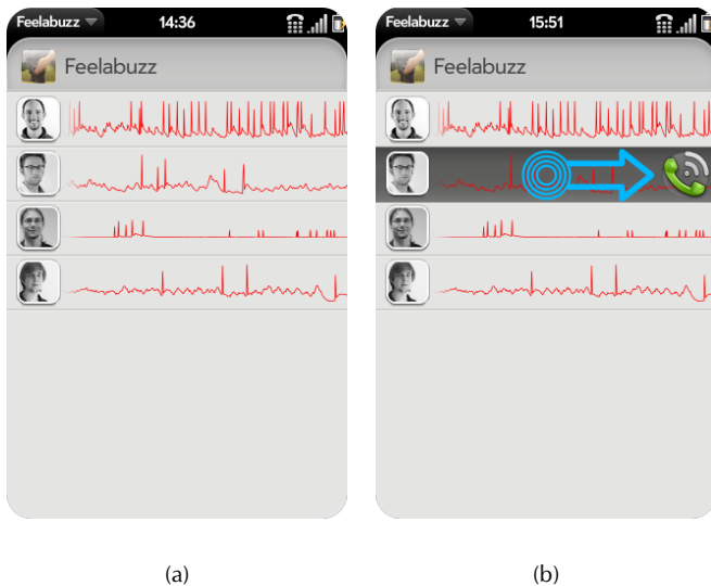
Figure 4.5. Screenshots of the WebOS dialer application. The interaction is illustrated in (b): the activity of a remote contact is rendered to the vibration motor when this contact is touched (blue circle). Additionally, a call icon is displayed. By moving the finger and releasing it on the icon, a call to the contact is initiated. Pictures by Sebastian Hammerl
