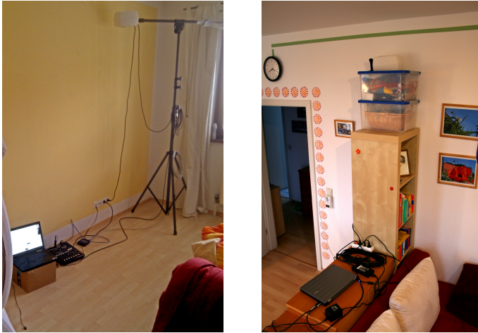
Figure 5.9. Two setups of upstairs by participants of our study (cf. Chapter 6). To get the speaker as close to the ceiling as possible, either a 165–350 cm speaker stand or available furniture was used. Photographed by the participants.
