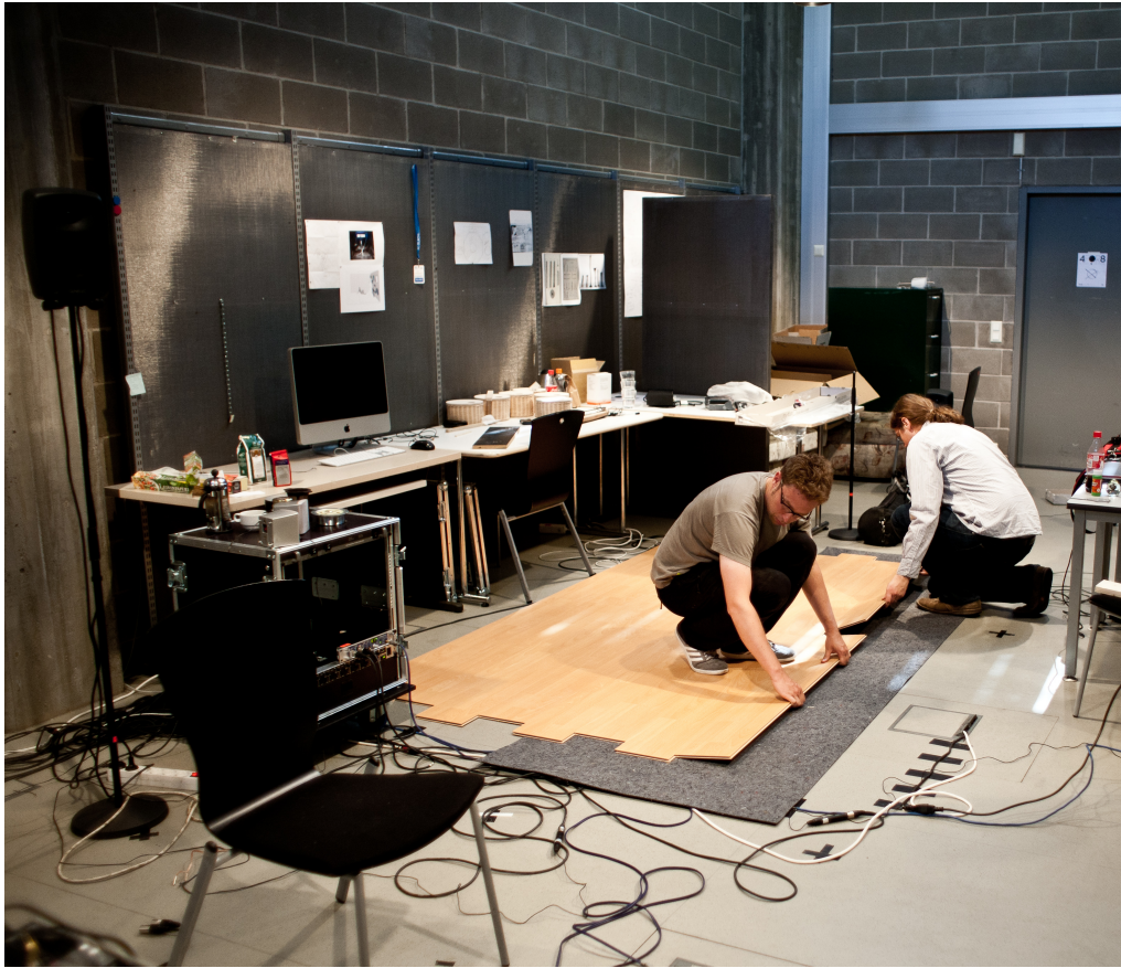
Figure 5.6. Construction of one of the upstairs test setups. The partial felt padding can be seen. Photo by René Tünnermann
