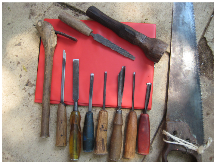
Figure 5.10: From left to right: anchô , knife, three different wood chisels, three different coivas and handsaw. From up to down: batedor and file (2008).
